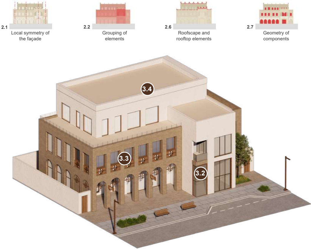
Axonometric view showcasing an example of the application of compositional rules for contemporary style low-rise mixed-use buildings.
