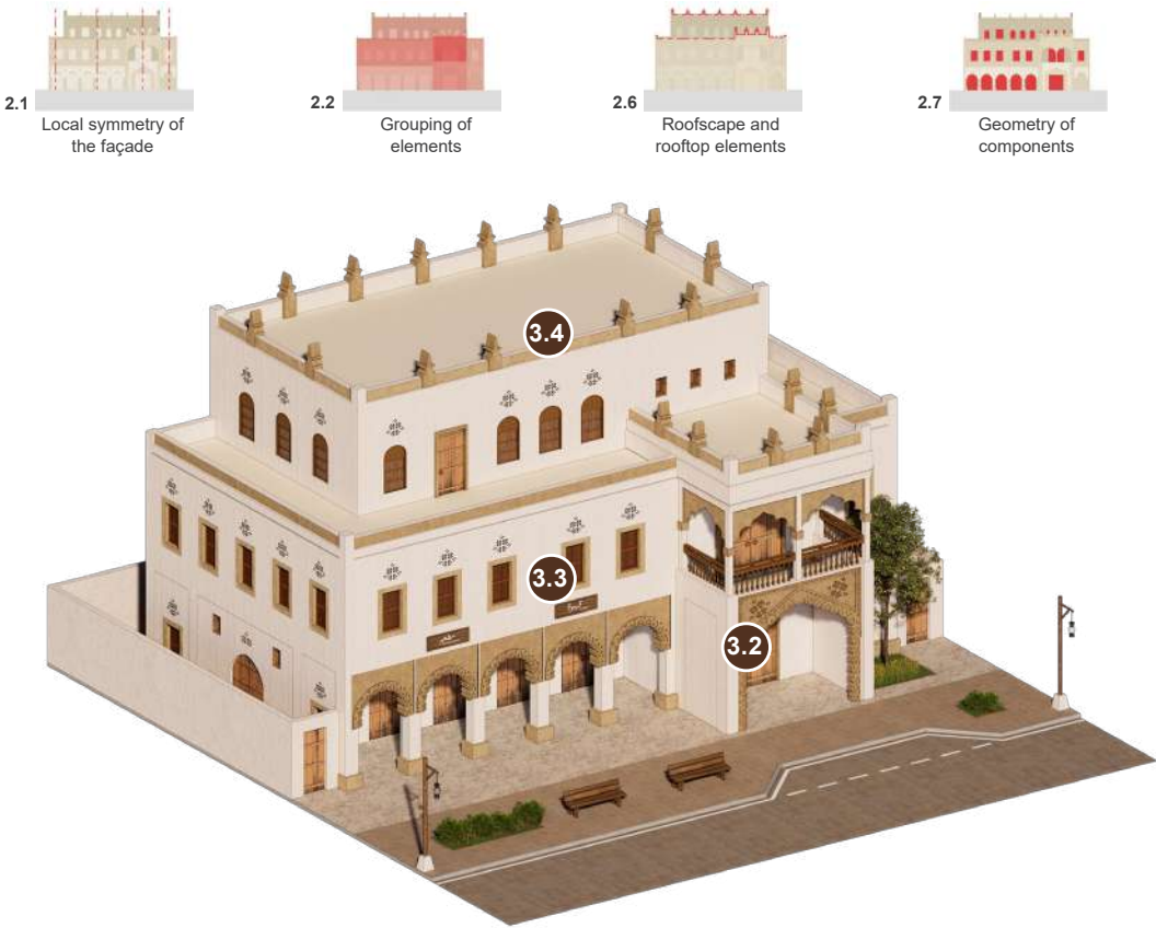
Axonometric view showcasing an example of the application of compositional rules for traditional style low-rise mixed-use buildings.
