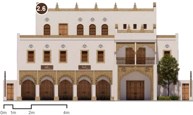
Elevation view showcasing an example of the application of compositional rules for traditional style low-rise mixed-use buildings.
