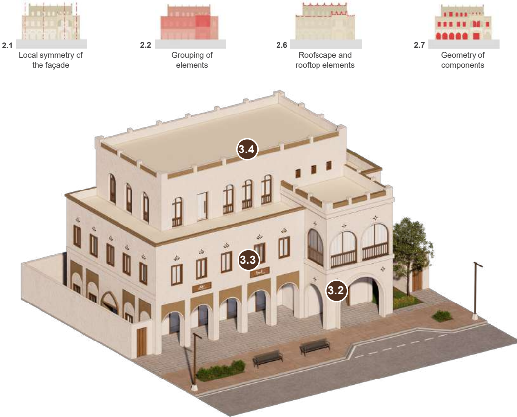
Axonometric view showcasing an example of the application of compositional rules for transitional style low-rise mixed-use buildings.
