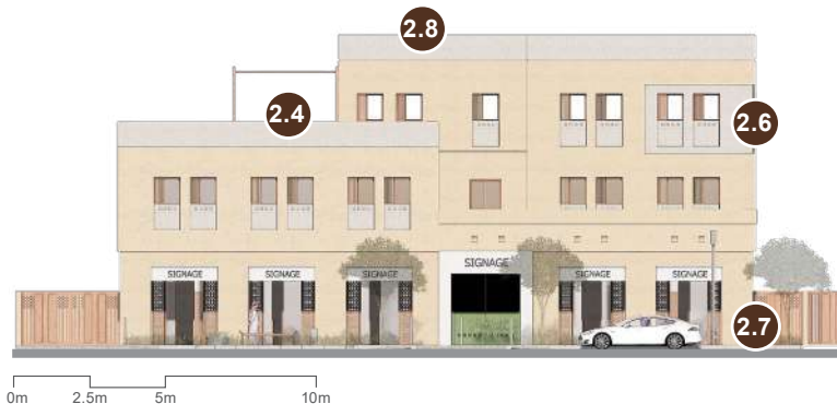
Elevation view showcasing an example of the application of compositional rules for contemporary style low-rise mixed-use building
