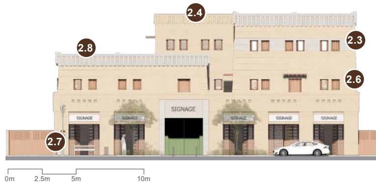
Elevation view showcasing an example of the application of compositional rules for traditional style low-rise mixed-use building
