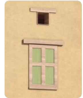
2 Timber framed and shuttered windows with high level vents.
