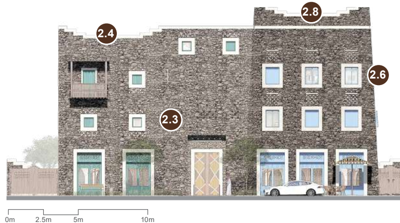
Elevation view showcasing an example of the application of compositional rules for traditional style low-rise mixed-use building
