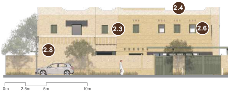
Elevation view showcasing an example of the application of compositional rules for traditional style building
