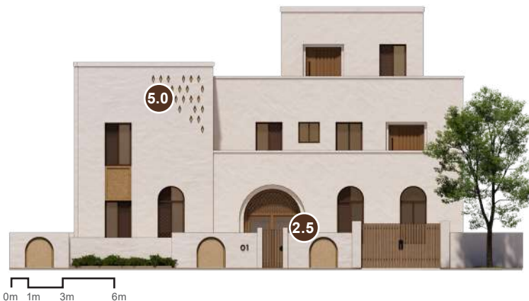
Elevation view showcasing an example of the application of compositional rules for contemporary style residential villa.
