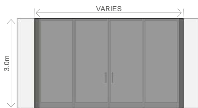
Vehicular access gate
