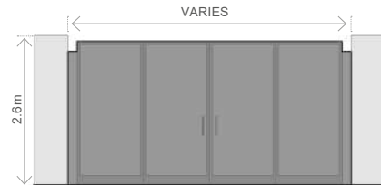
Vehicular access gate
