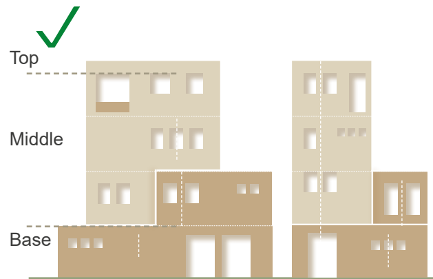
FIG. 30 Variation of moderate sized openings with localized symmetry should be encouraged. Max. 30-50% openings. Loggias and terraces incorporated in facade design. Privacy for neighboring plots
