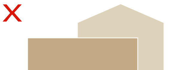
FIG. 25 Large monolithic building blocks, non contextual roof profiles should be avoided
