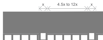
Parapet Type C
